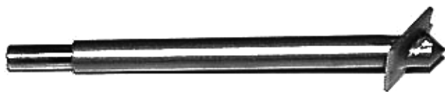
Fig. 1. The propeller mounted to the rheometer used for agitating and measuring shear stress after adding alginate to the water. Made by Rheologica AB, Lund, Sweden. The propeller, positioned 6 mm above the bottom of the rheometer cup, had the following dimensions: length 99 mm, bar diameter 7.5 mm, vertical blade height 10 mm, blade angle approx. 48° and propeller diameter 18 mm.
